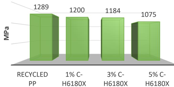
The flexural modulus of the recycled PP is not strongly affected by the presence of Calprene H6180X
