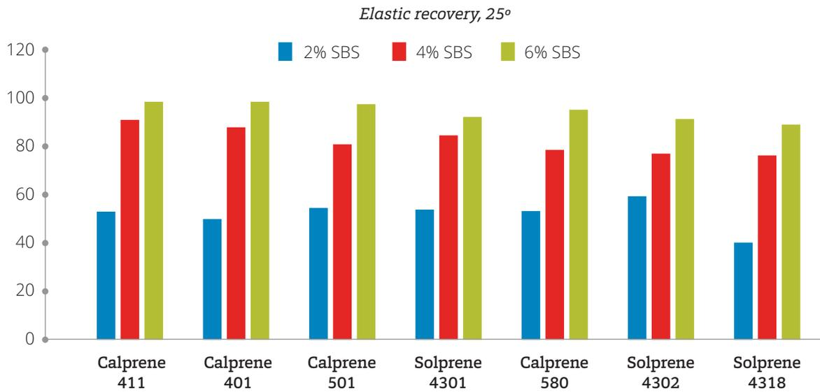
Figure 8. Elastic recovery 25° HMA with SBS
