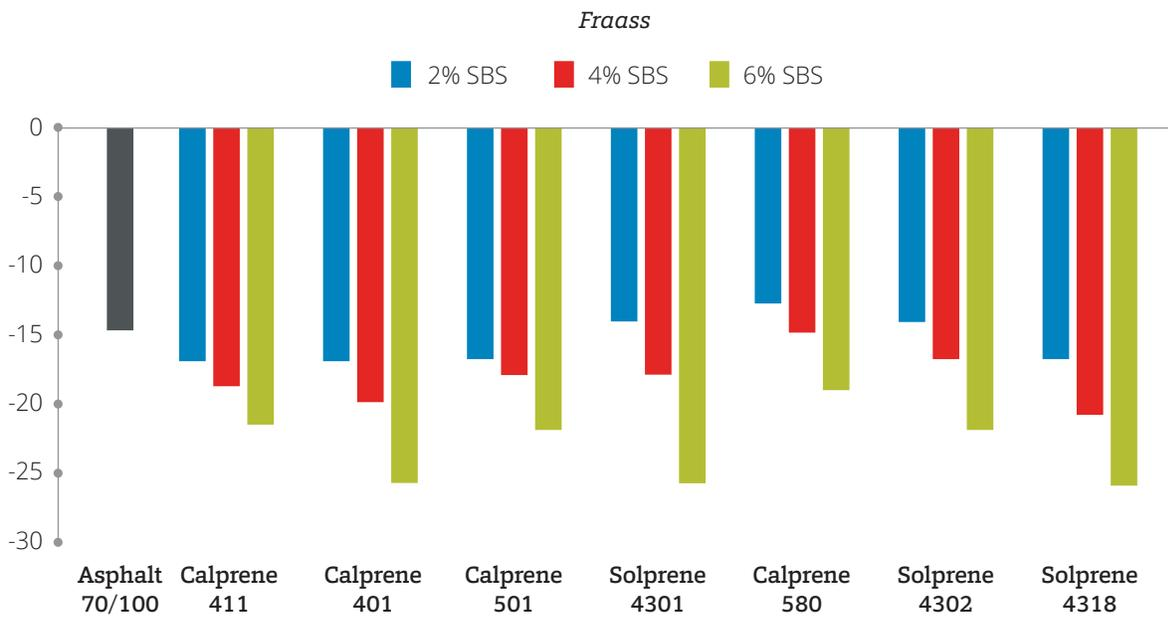
Figure 7 . Fraass HMA with SBS
