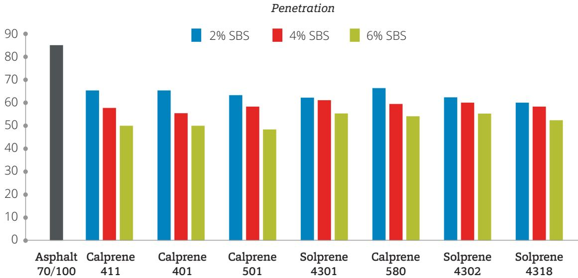
Figure 6. Penetration HMA with SBS
