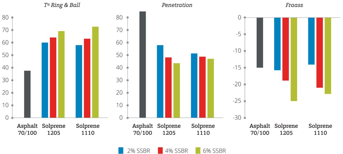
**Figure 2. R&B temperature HMA with SSBR**
