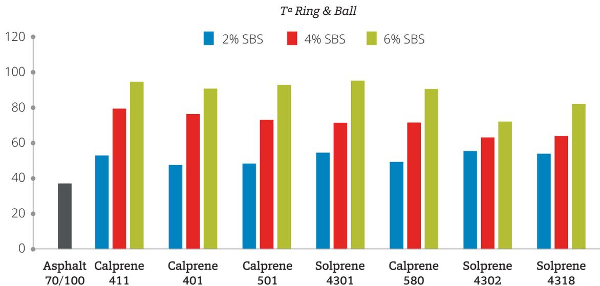
**Figure 5. R&B temperature HMA with SBS**
