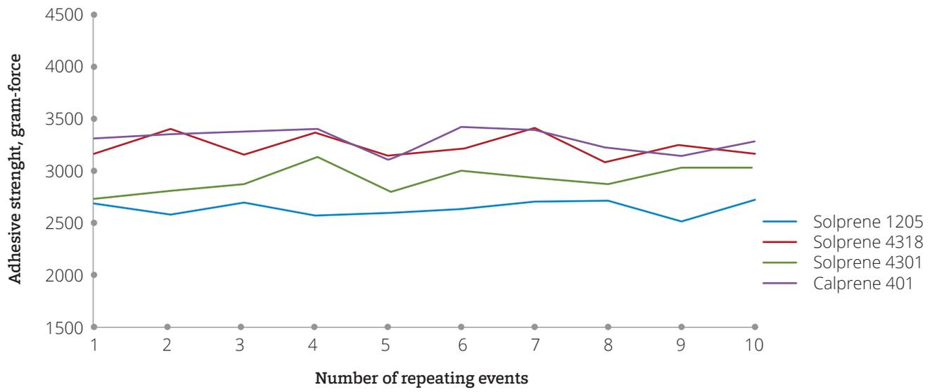
Figure 13. Adhesive strength from asphalt residual
